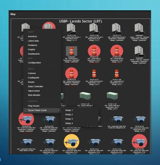
Allows cycling of device power remotely. PC / Modem cycle reboots both of those devices. Switch Cycle will reboot all cameras. Fan Cycle is temperature controlled and acts as the thermostat locally in each device to control airflow.
