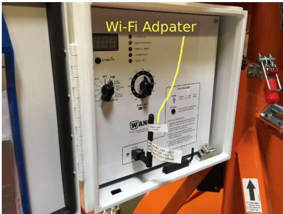
Figure 3.2: The USB Wi-Fi Adapter That Is Plugged In
