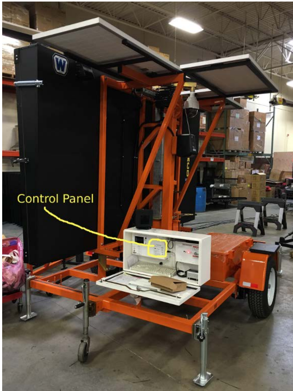
Figure 2.3: Control Panel of Wanco Message Trailer
