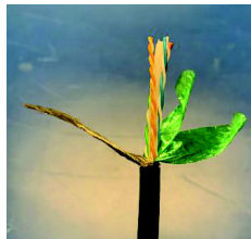
Figure 4: Cutting the Center Spline and Trimming the Shielding
