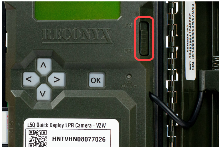
Figure 6: L5Q Power Switch
