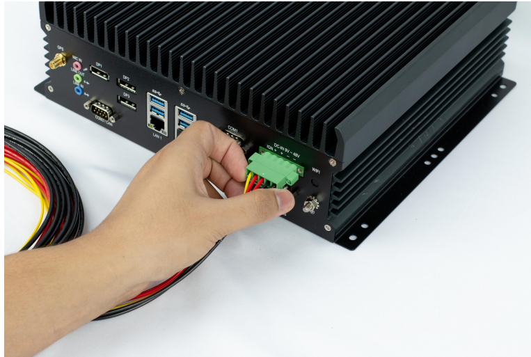
Figure 3: Wiring Harness to VLP Box
