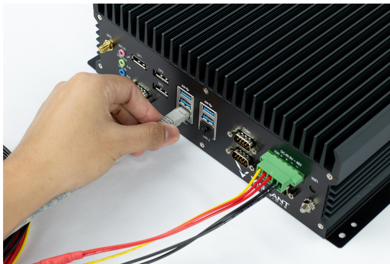
Figure 4: Ethernet Cable to VLP Box
