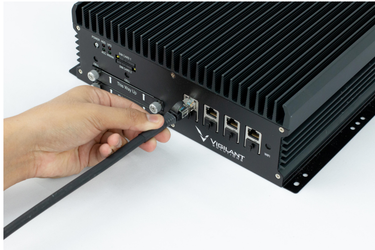
Figure 5: Camera Cable to VLP Processor
