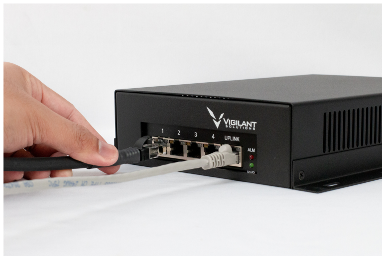
Figure 9: Camera Cable to PoE Injector
