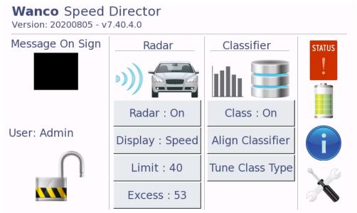
Display will show oncoming vehicles speed. When over speed the unit will flash and if above excess speed will blank
