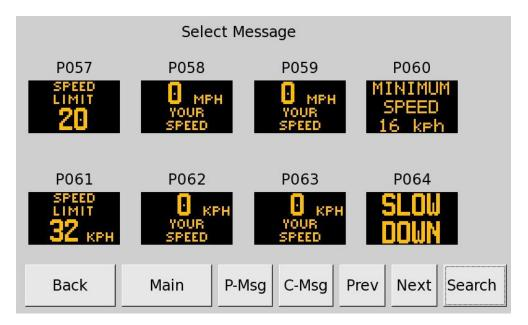
The sign displays message **P057**: **SPEED LIMIT 20**. If the speed of the approaching vehicle is below 20 MPH, the message **P058** is displayed (with the actual speed) without flashing, and if the actual speed is within the range 0 to 15 MPH over the posted limit, the message **P059** is displayed that is the actual speed flashing. However, if the speed exceeds this range, the excessive speed message **P064** (**SLOW DOWN**) is displayed.
