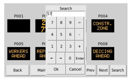
Touch **OK** and get the screen shown below that shows all default messages for the radar speed trailer function, i.e., the messages **P057**, **P058**, **P059**, and **P064**.
