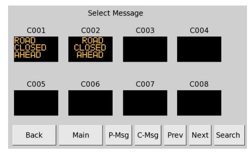
For the time being, we touch P-Msg button and obtain **Select Message** screen with pre-programmed messages as shown below. Using **Prev** and/or **Next** buttons (as explained below), we can reach any P-Msg. In addition, if we know the message code, we can get to it using the **Search** button.
