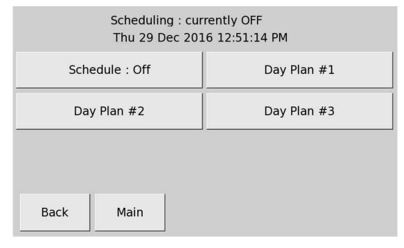
The first thing before we start is to make sure that the day of the week, the date, and the time is correct on the sign. We will work on **Day Plan #1** to illustrate how to set that up and how it might be used. We have already pre-programmed some messages in there to make our explanation shorter and showing the essential points. As shown below **Day Plan #1** has everything blank.
