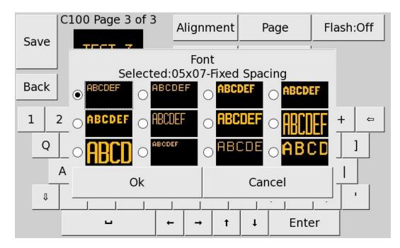
You also can choose either **flash-on** or **flash-off mode** for any of the lines of your message. Page 3, after the modification performed, is shown below.
