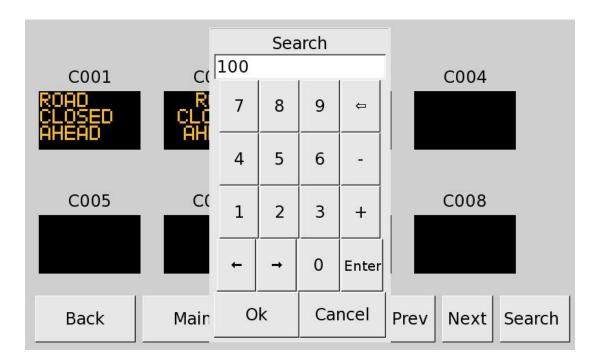
Our **C100** message comes up in the **Select Message** screen shown below and it is selectable/can be activated from this screen by touching. Note that this screen shows 8 slots with C-messages from C100 to C107. Thus, the **Search** button can be used to reach groups of messages starting with C030, C040,..., etc. In these 30-series or 40-series messages, we can preload messages associated with specific tasks, specific traffic conditions, specific projects, etc.
