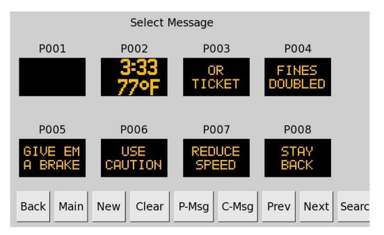
In this screen you can find (using the buttons **P-Msg**, **C-Msg**, **Prev**, **Next**, **Search**) the messages that you want to include in your new group. Once you touch the desired message, the **Select Message For Group** screen appears with the previously blank space filled up with the selected message. In the same way, you insert next messages into your group. Also, using **New** button in **Select Message** screen you can compose any message that you would like to add to your group.
