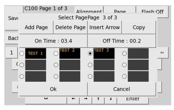
Touch **OK** to obtain the *quick message composition screen*. Touch **Alignment** and in the Alignment window select **Center** (the other choices are: **Left** and **Right**) and **Middle** (the other choices are: **Top** and **Bottom**). Touch **OK**, **Save**, and **Activate This Message** on the consecutive screens as they show up. Following the same procedure, you can align the text on each page of your multi-page message.
